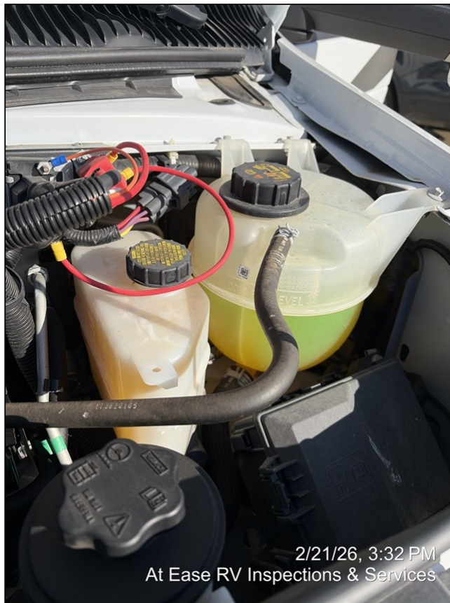
14.6 Item 1 (Picture) Coolant reservoir
