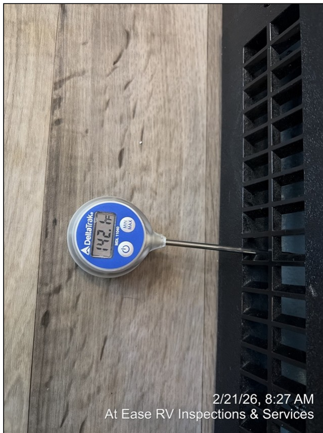
21.7 Item 1 (Picture) Output temp in kitchen area
