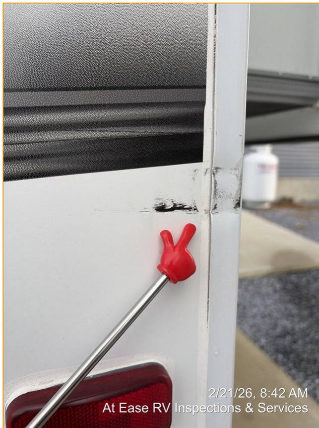
6.0.D Item 1 (Picture) Scratch/dent at rear wall joint
